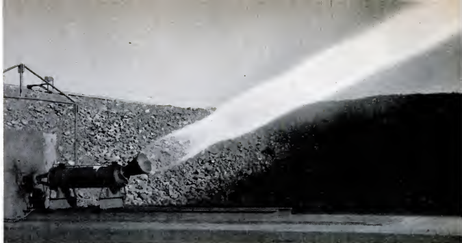
POWERFUL SOLID-FUEL ROCKET MOTOR , the type used in Polaris, is tested at Aerojet's plant near
